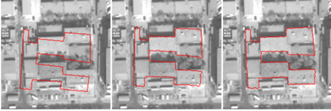
Figure 5.19: Successful matching with a distant initialization and insertion of the exogenous DSM in the energy functional (GVF model for the image, Chan and Vese model for the DSM).
