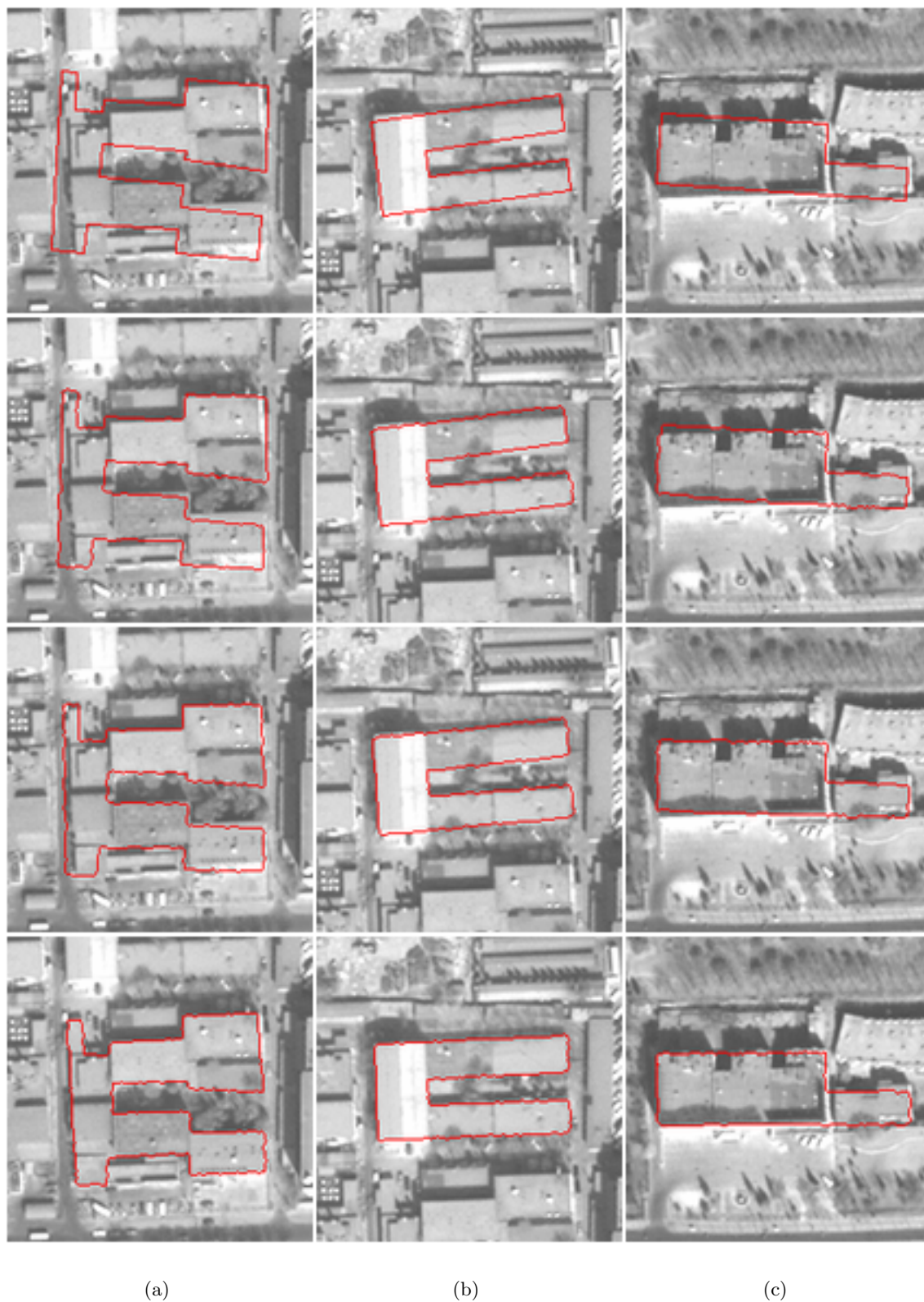
Figure 5.13: Sensitivity to initialization: segmentation with an active contour based on the contour information (GVF) and with the shape constraint.
