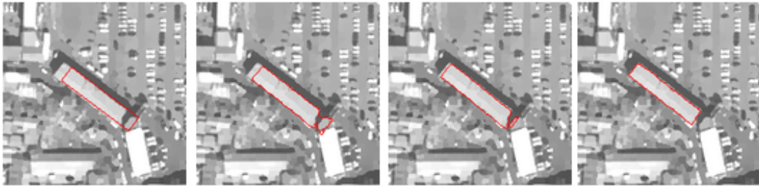
Figure 5.21: Segmentation with a spatio-temporal variation of the shape constraint and the Bayesian model ( \lambda_{min} = 3 , \lambda_{max} = 30 , d_0 = 7 ).
