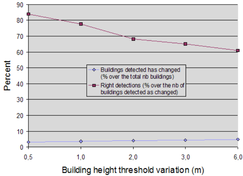
Figure 7.6: The method's success in relation to thres_{build} . The rate of buildings correctly detected as having changed is shown in red. The blue curve represents the rate of buildings detected as having changed in relation to the total number of buildings on the map. thres_{filled} = 65\% and thres_{flat} = 1.5m .
