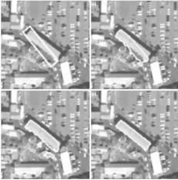
Figure 5: Convergence sequence (from top to bottom and left to right) illustrating the matching process with a flexible shape constraint ( 5 < \lambda_{flex} < 30 , \lambda^d = 0 ).
