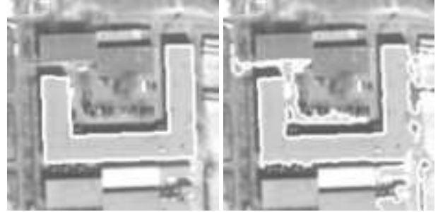
Figure 2: Matching without shape prior. Left: initial state close to the desired solution. Right: result without shape prior, “leak” of the active contour.
