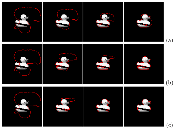
Fig. 2. Segmenting curve evolution from left to right: comparison between constant and spatio-temporal shape prior weight. (a) \lambda = 100 , (b) \lambda = 10 (c) spatio-temporal function with d_0 = 10 , \lambda_{min} = 20 and \lambda_{max} = 100 .
