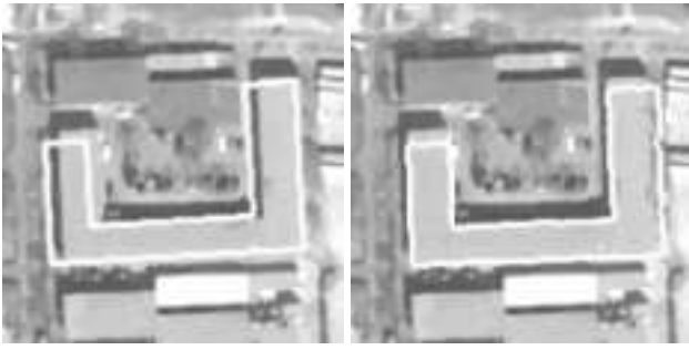
Figure 8: Matching with flexible shape prior and DSM fusion and a locally mistaken cartographic object ( 5 < \lambda_{flex} < 30 , \lambda^d = 0.75 ). Left: initial state derived from the map. Right: unsuccessful complete matching result.
