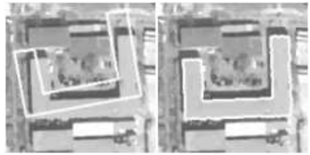
Figure 6: Matching with DSM fusion ( \lambda_{flex} = cst , \lambda^d = 0.75 ). Left: initial state. Right: successful matching with DSM fusion.
