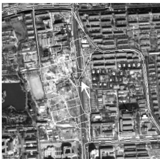
Fig. 1. Tsinghua University area, Beijing, China: GIS road layer displayed in white (1996) registered by global affine transformation on a Quickbird satellite image (2002). The white arrow points some changes.
