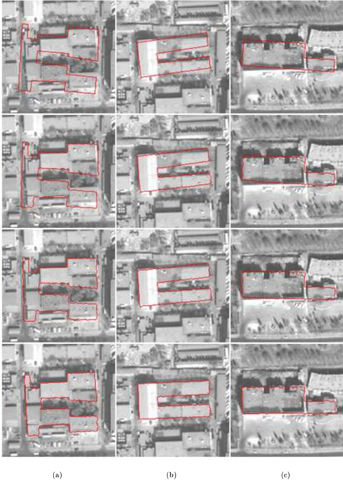
Figure 5.13: Sensitivity to initialization: segmentation with an edge-based active contour (GVF) and with the shape constraint.
