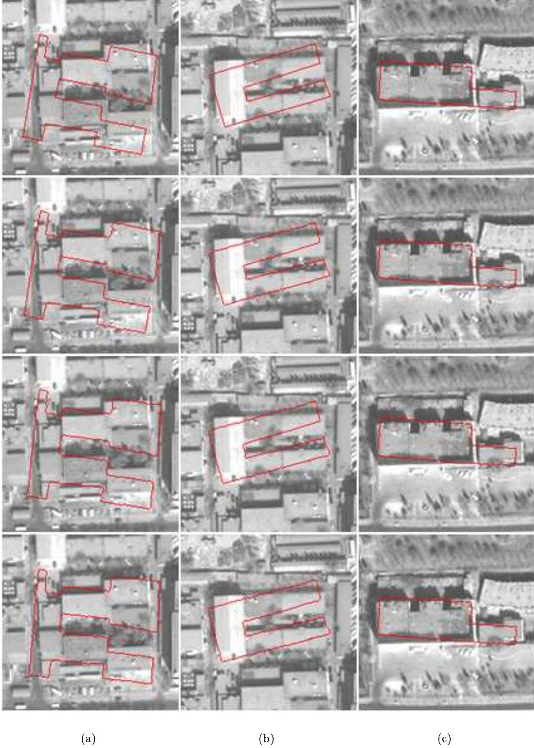
Figure 5.14: Sensitivity to a distant initialization: segmentation with an edge-based active contour (GVF) and with the shape constraint.
