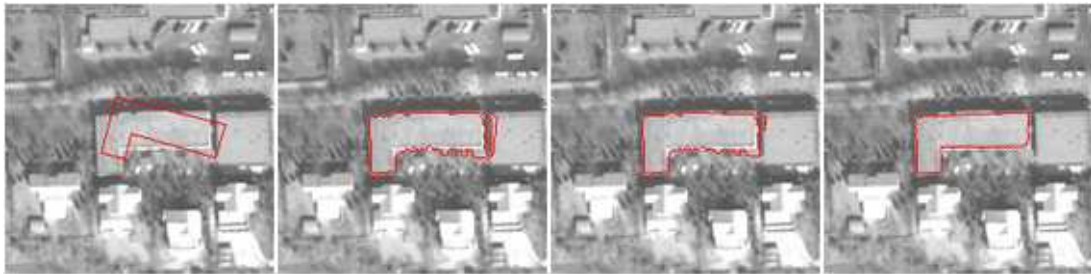
Figure 5.22: Segmentation with a spatio-temporal variation of the shape constraint and the Bayesian model ( \lambda_{min} = 27 , \lambda_{max} = 70 , d_0 = 7 ).
