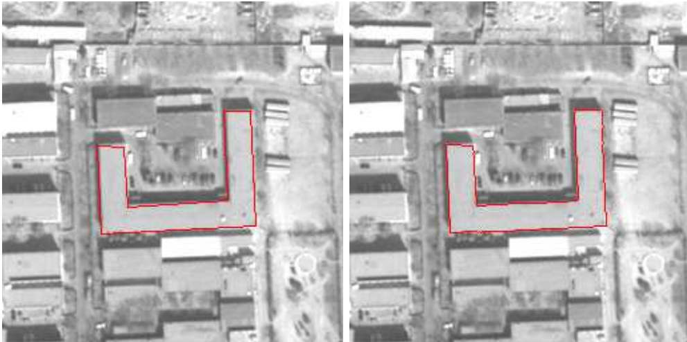
(a) Initial map-to-image superimposition without active contours matching
