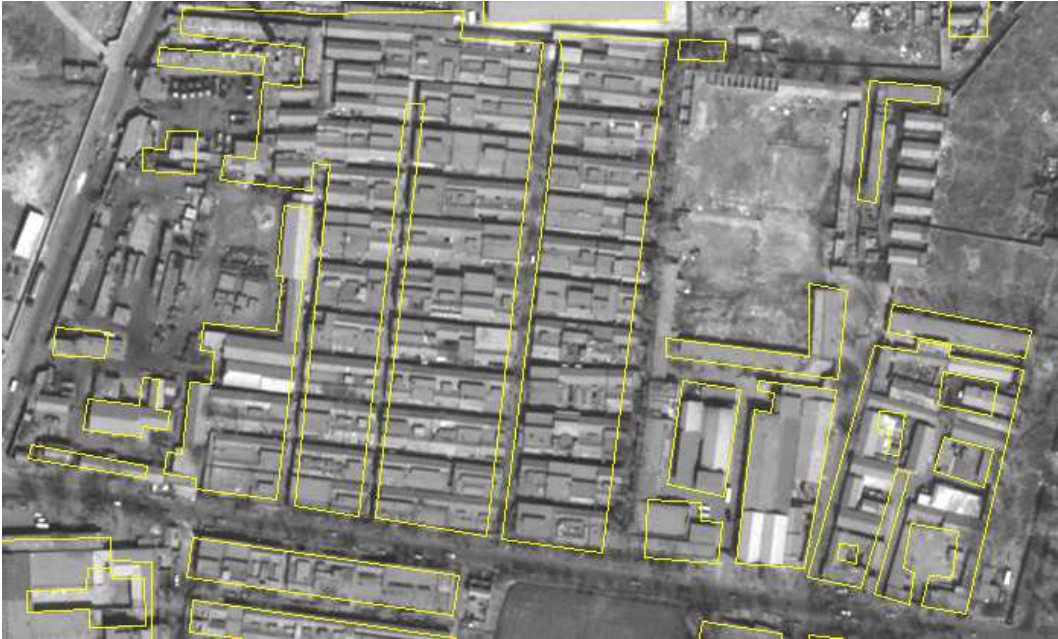
Figure 2.4: Superposing of a map of the constructions (yellow polygons) with a satellite image illustrating the generalization effect: a single cartographic polygon encompasses numerous adjacent buildings.
