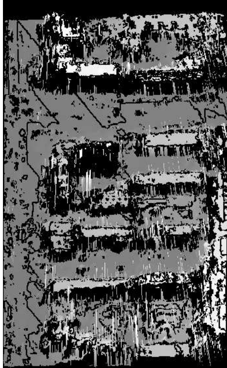
Figure 3.21: DSM orthorectified with a pitch of R = 0.65 m and \varepsilon_{corr} = 0.4 .
