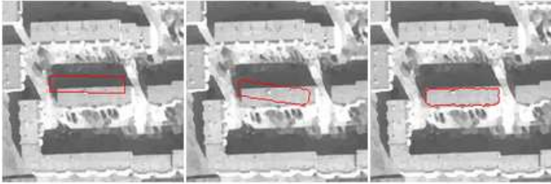
Figure 5.18: Successful matching with a distant initialization and insertion of the exogenous DSM in the energy functional (Bayesian model for the image, Chan and Vese model for the DSM).
