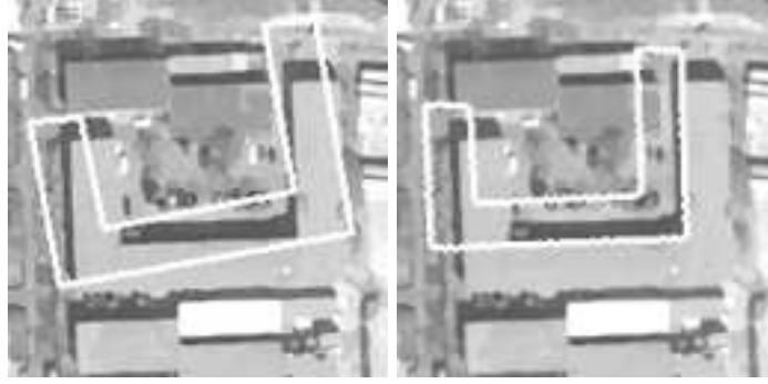
Figure 5.16: Failed matching with a distant initialization and the Chan and Vese model (no incorporation of the DSM).
